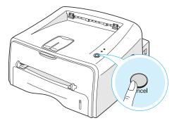
The printer will finish printing the page that is moving through the printer and delete the rest of the print job. Pressing **Cancel** cancels only the current job in the printer. If more than one print job is in the printer memory, **Cancel** must be pressed once for each job.
